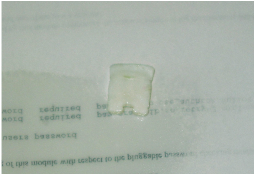
Figure 9: Adhesive sprayed on front pointing half of elastomer. Contrast and brightness were adjusted with Gimp for visibility.
